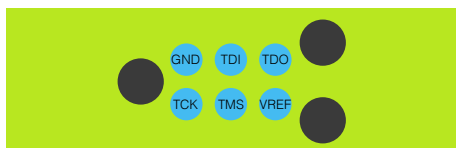
Figure 56: Foot print for tag-connect header
