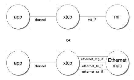
Figure 1: XTCP task diagram
