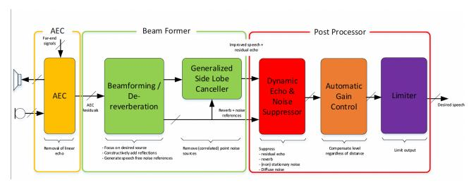
Fig. 3.1: Voice processing pipeline
