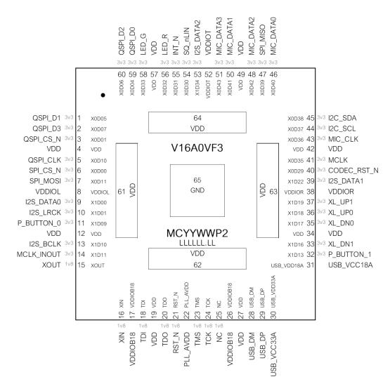
VDDIOT, VDDIOL and VDDIOR must be connected a 3V3 supply. VDDIO18 must be connected to a 1V8 supply, and all VDD pins must be connected to a 0V9 supply. All package paddles (pins 61 through 65) must be connected. It is advised to place a via under each paddle to connect it directly to a PCB supply plane.
