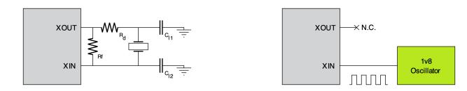
Fig. 6.1: Crystal oscillator or clock input configurations
