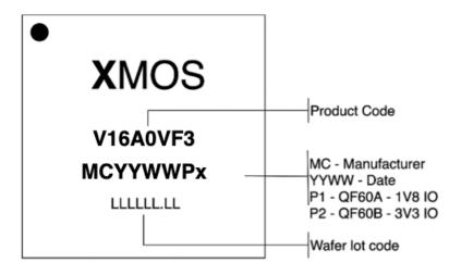
Fig. 8.2: XVF3800 Package Marking
