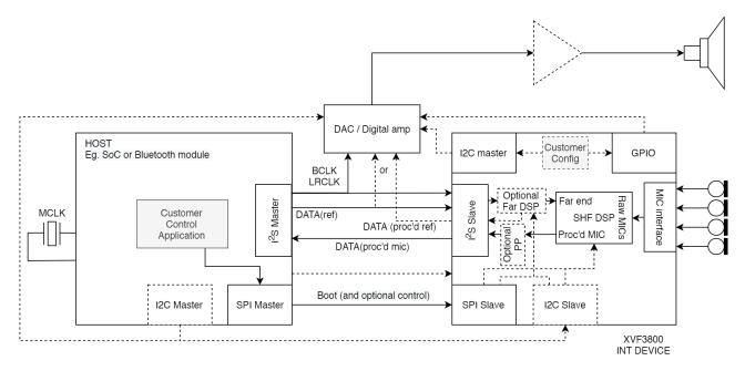
Fig. 2.2: Functional block diagram of XVF3800 in INT-device configuration
