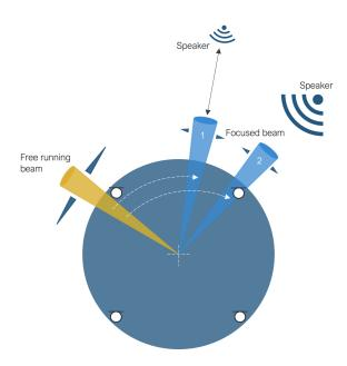
Fig. 3.2: Beamformer Operation
