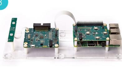
Screw longer spacers into place on top of RPi and then push Pi HAT onto RPi. Use plastic screws to fix Pi HAT board on top of the RPi.
