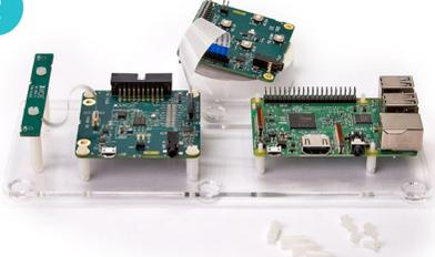
Fix Raspberry Pi to plastic stand using shorter plastic spacers to support the Raspberry Pi.
