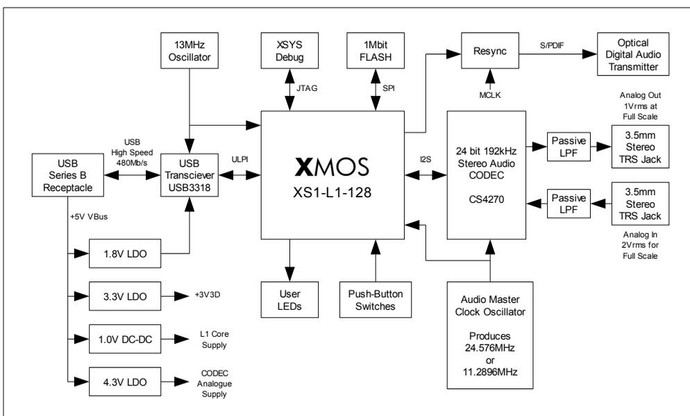
The XS1-L1 event-driven processor communicates with the USB host via a ULPI USB transceiver at the 480Mb/s high-speed rate. The XS1-L1 controls the streaming of audio data over the USB connection and direct I<sup>2</sup>S interface to the audio CODEC. Multiple additional functions (e.g. Mixers/DSP etc.) can be implemented by modifications to the standard software.
