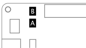
The LEDs are connected to two bits of port 32A as shown in the port map. Setting the relevant bit high will turn the LED on.
