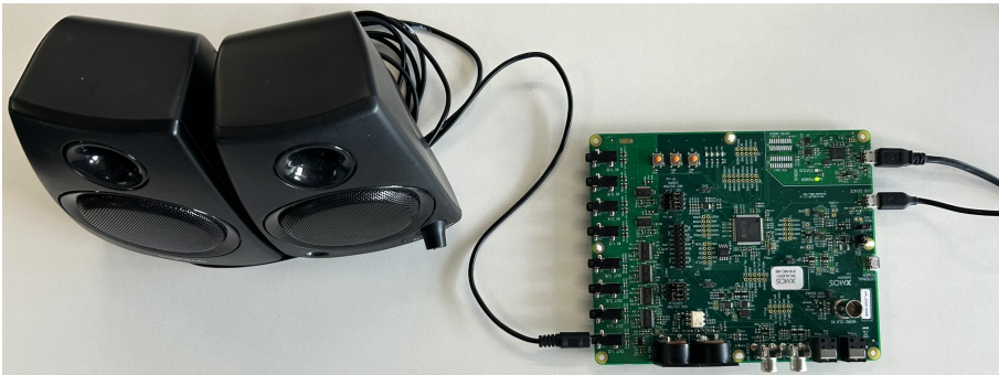
Fig. 1: XK-AUDIO-316-MC-AB with both USB cables connected and a pair of speakers connect to OUT 1/2
